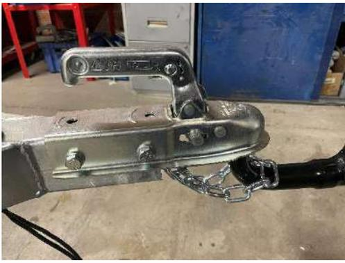
**BOITIER D'ATTELAGE BIEN VERROUILLÉ AVEC CHAÎNE DE SECURITÉ EN POSITION CORRECTE**
